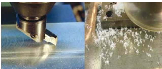
Figure 1: Single fly cutting action
